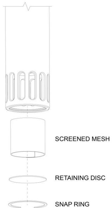
**Figure 4-1:** Screened Intake Components
